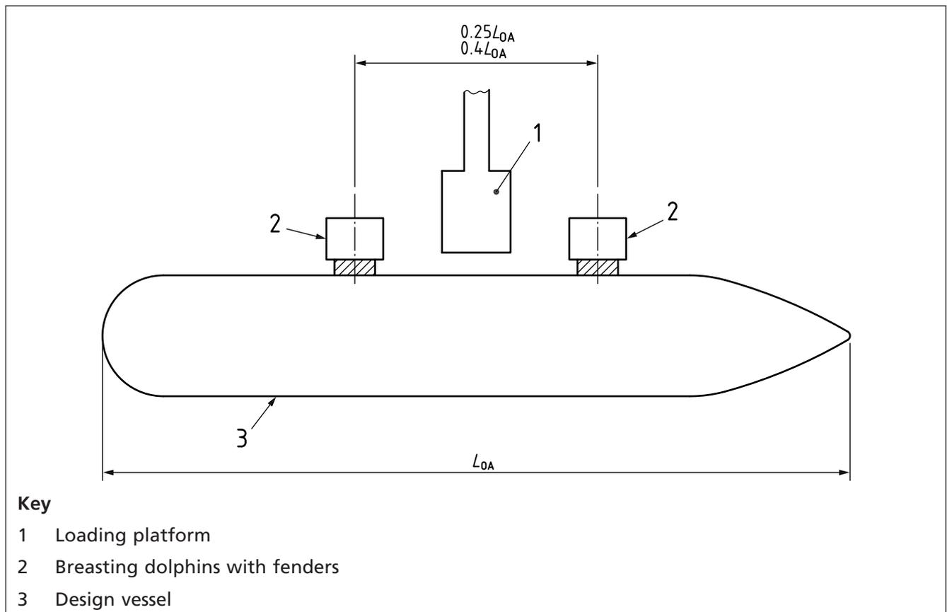
Figure 5 Fender layout for five island berth
