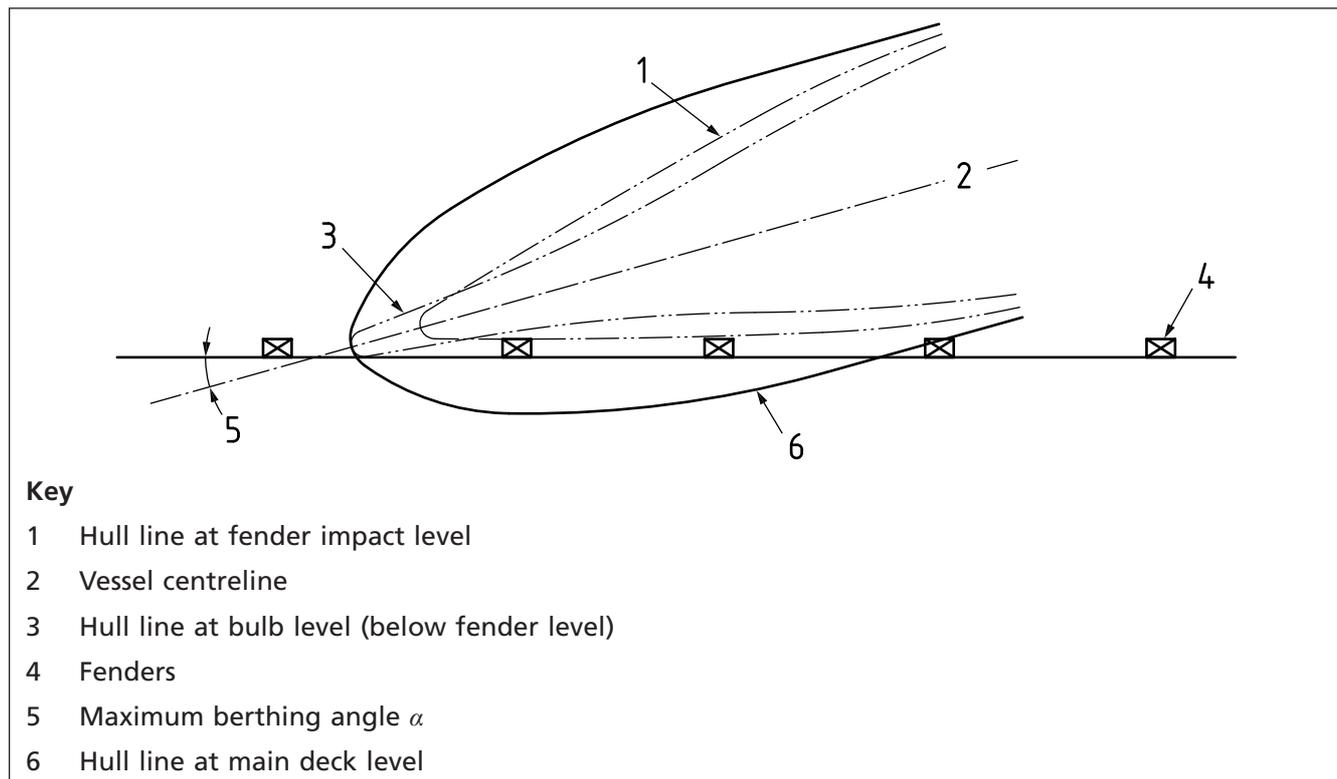
It is generally impracticable to provide a fendering system to safeguard the berth structure against accidental head-on or steeply-angled impacts. The designer should therefore establish a maximum safe value of the berthing angle that can be achieved whilst optimizing both the fendering system and the substructure layout.
