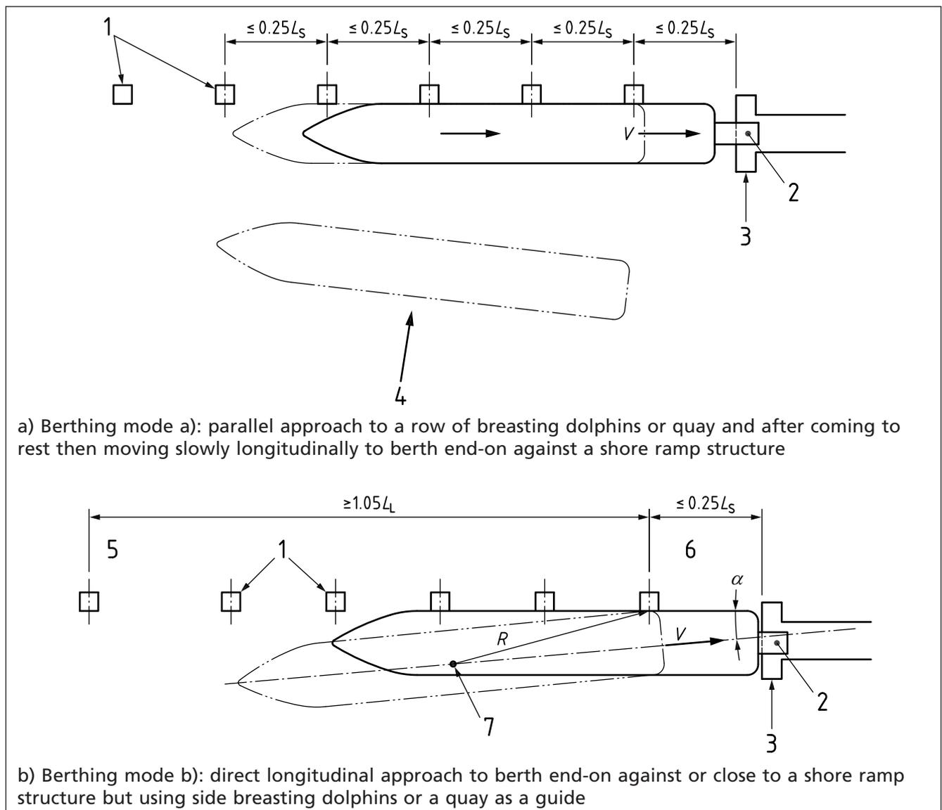
Figure 7 Ferry and Ro-Ro vessel berthing (2 of 2)
