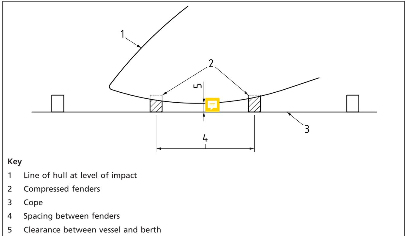
Figure 3 Fender layout on a continuous quay
