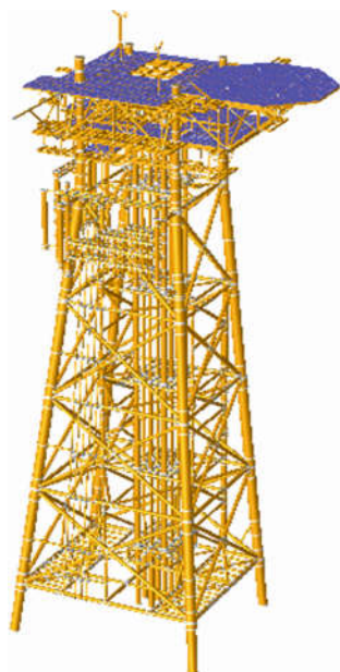
Fig. 1. Model of Dong Do wellhead
