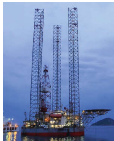
Fig. 1. Jack up rig in transit condition
